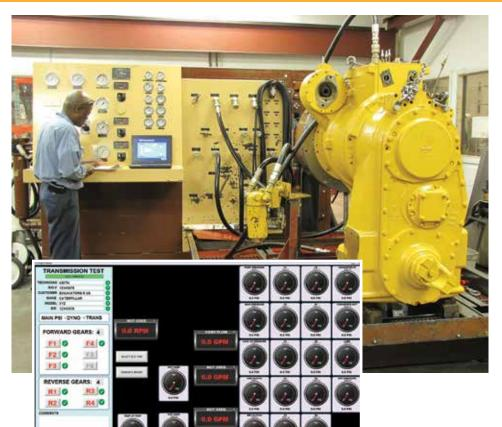
TRC's dynamometers are complete with computerized Data Acquisition programs that sample three data points every second.
